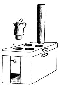
of ten to twenty. It was almost an indispensable article with such large companies. It is a round-cornered box, twenty-one inches long by twenty wide, and thirteen inches high, with a slide in the front end to admit air and fuel. The bottom is fixed to the body; the top removes, and
